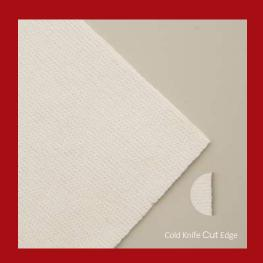
Valutek's standardweight polyester wiper is constructed from 100% continuous filament polyester in a double-knit, no-run, interlock pattern with cold knife-cut edges. This wiper is a clean and moderately absorbent wiper with low levels of particulate and extractable counts.
